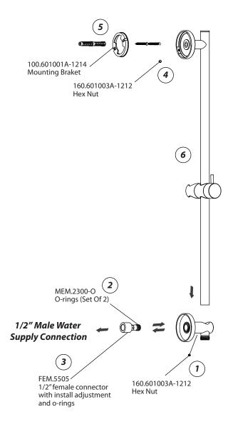
**1.** Loosen & remove the hex nut using 1.5mm Allen key.
